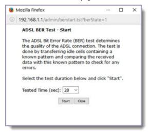
2. In the **Tested Time** field, select the duration in seconds and click **Start**. Options range from **1 second** to **360 seconds**. The test transfers idle cells containing a known pattern and compares the received data with this known pattern. Comparison errors are tabulated and displayed. To stop the test, click **Stop**.
